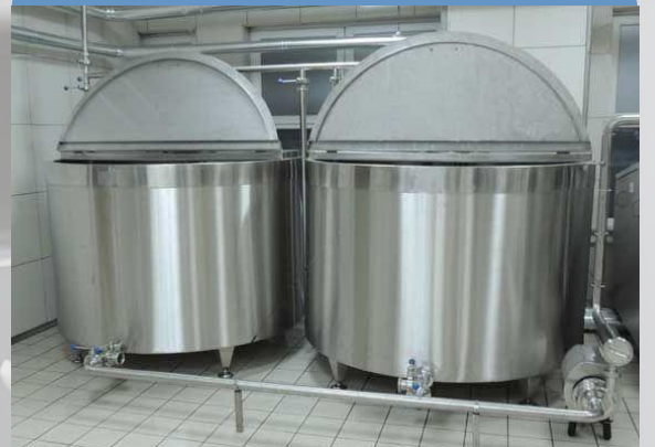
SÜT PİŞİRME KAZANI (MILK COOKING BOILER)
